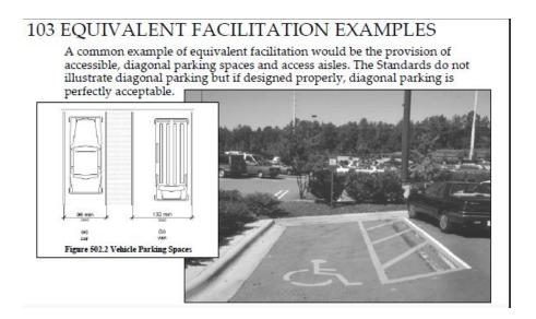
And another one showing for diagonal parking. The code doesn't really address these specifically, but these can be done as equivalents using basically the same dimensions.
